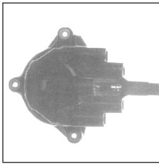
M4 distributor cap - straight fitting 18mm
